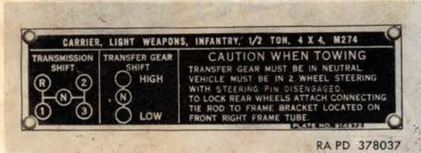
Figure 4. Instruction plate located on top of platform at right of driver.
