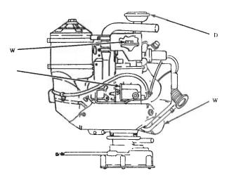
OE/ Crankcase Oil Fill HDO and Level Gage (See key) (Check level) (C)
