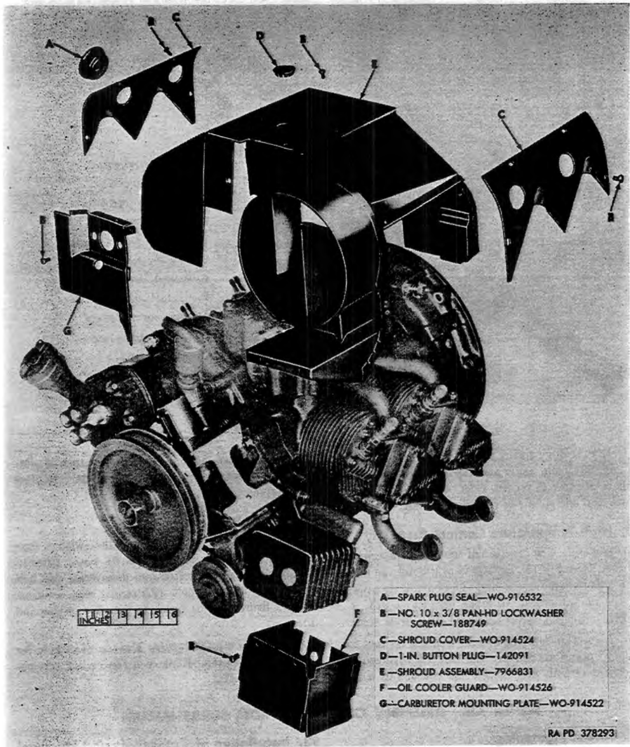
Figure 66. Engine shroud components—Exploded view.
