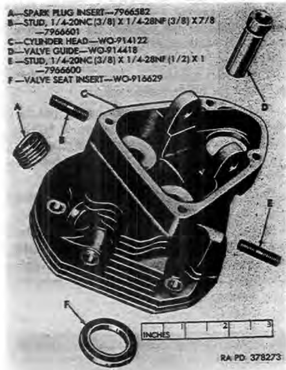
Figure 46. Cylinder head—Exploded view.
