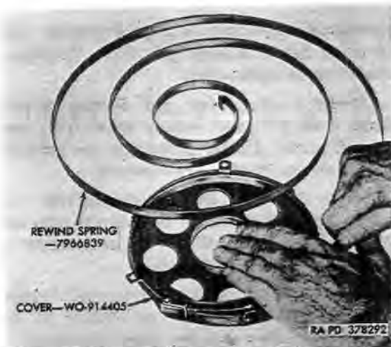
Figure 65. Unwinding starter rewind spring from cover.
