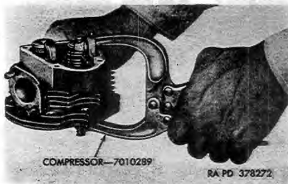
Figure 45. Compressing valve spring, using compressor 7010289.
