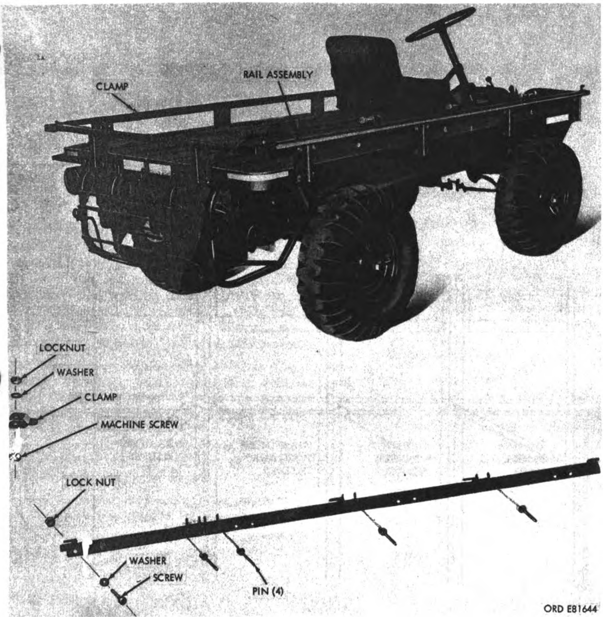
Figure 8-4. Location of rail assembly, machine screws, flat washers, and self-locking nuts.
