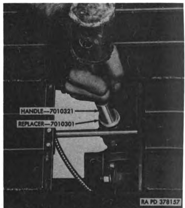
Figure 2-91. Installing front steering bellcrank bearing with replacer 7010301—M874A8 through M874A4.
