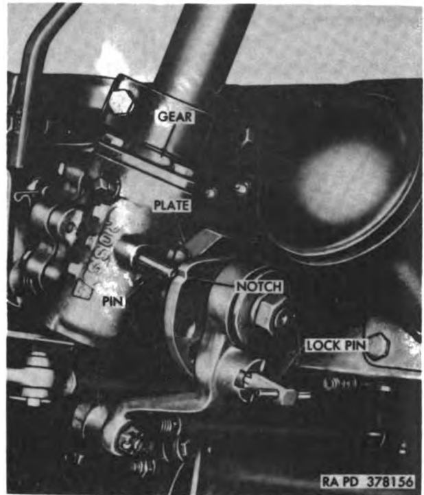
Figure 2-87. Position of steering gear, locking plate, and lockpin at final adjustment of steering system.
