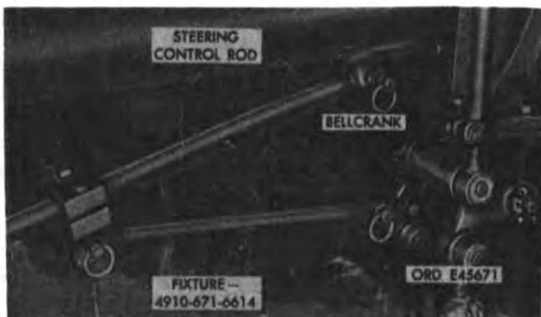
Figure 2-90. Special fixture 4910-671-6614 connected to bellcrank and steering control rod.
