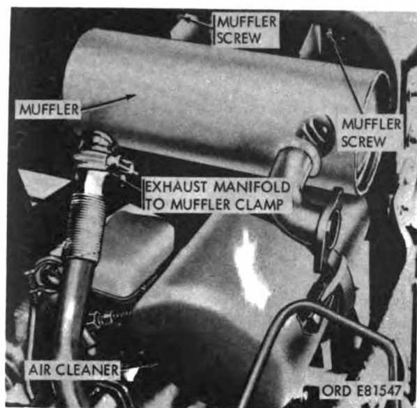
Figure 2-1. Location of possible exhaust leaks.
