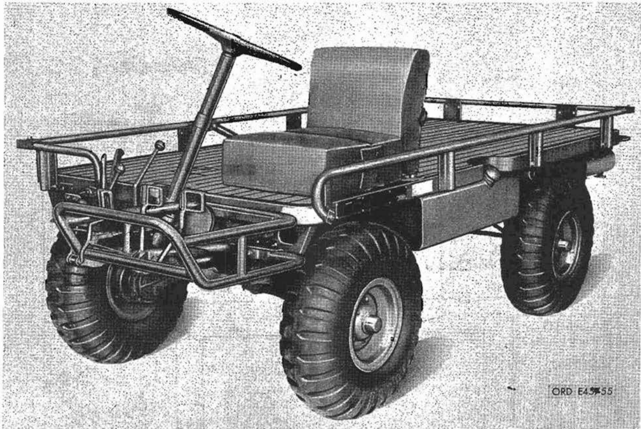
Figure 1. Left front view of 1/2-ton, 4 x 4, Platform Utility Truck - M274.
