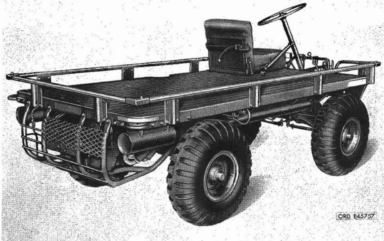
Figure 3. Right rear view of 1/2-ton, 4 x 4, Platform Utility Truck - M274.
