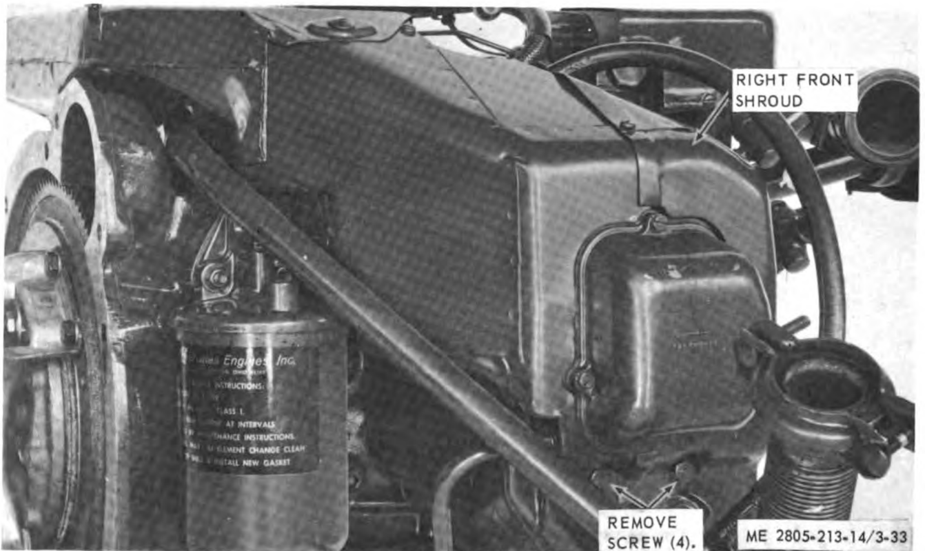
Figure 3-33. Left front, left rear, right front, and right rear shrouds, removal and installation.
