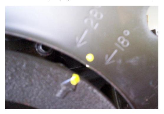
Turn fan drive pulley clockwise (much smoother and precise using a crescent wrench)
