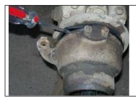
Use a screwdriver to pry the outer end of the rubber boot out of the slot in the knuckle housing. Make sure you have a catch pan, there should be oil here.
