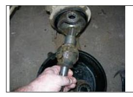
Now you can slip the axle out. Don't loose the spacer on the inner axle, and be careful, sometimes worn axle joints will come apart when you pull them out.
