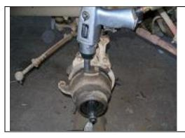
Now remove the nuts holding the top and bottom kingpins in the knuckle housing. There should be sheet metal locks under the nuts, but they were missing on this mule.
