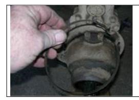
Remove the band completely. Don't forget to put the nut back on the screw for safekeeping!
