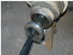
If you are only changing the hub seals, use a seal puller to remove the old seals and install new ones.
