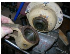
This is a good time to pry the lifting ring off the hub and clean everything up and install new O-ring seals. Use grease on the O-rings when you go back together to keep everything free. Don't leave the seals out, or dirt and water will enter your hubs
