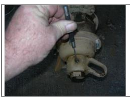
Now the fun part, use a long punch to remove the lock pin. It is supposed to be a 9/64" x 1 1/4" spring pin. No telling what you will find, and you may have to rotate the lifting ring to find the hole with the locking pin in it.
