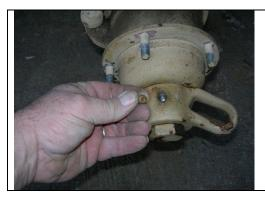
Next, remove the two 1/8" plugs. They should be brass with a straight screwdriver slot or an allen socket, but no telling what you might find. Whatever you have, they both must be removed.
