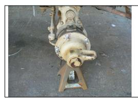
Sounds simple, remove the 5 lug nuts.....but sometimes the wheel is stuck to the hub and it may take lots of force with a dead-blow hammer on the back of the tire.
