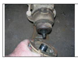
Once the nut is off, you can slip the hub off the axle.
