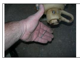
In this case it was a cut-off nail. That's about normal, that's what I find in about 9 out of 10 hubs! This does not work, because the nail will slide down into the hole in the lifting ring and then the ring won't turn....then somebody gets a long pry bar.....and you know the rest!
