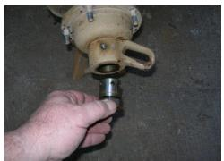
Once you have removed the spring pin, nail, wire, stick, whatever you find, you are ready to remove the retaining nut from the axle. DON'T try to remove the nut until you have removed the locking pin or know for certain that there is nothing locking the axle nut to the axle. A broken piece of spring pin can really screw-up the threads inside the nut (experience talking!)
