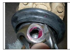
I put the twisted part at the top, where the boot does not flex as much.
