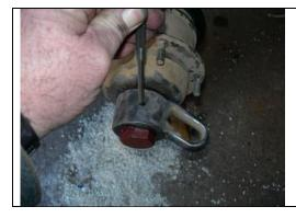
I use my large pinch to drive the pin flush with the nut.
