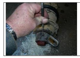
Then switch back to the smaller punch to drive the pin slightly below the nut until the lifting shackle will turn freely.
