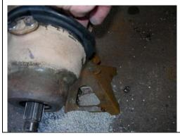
And use your hands to roll the boot into place in the groove on the knuckle. If you use a screwdriver, be careful not to poke a hole in the boot!
