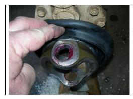
And be careful to tuck the end down where it can't damage the boot.
