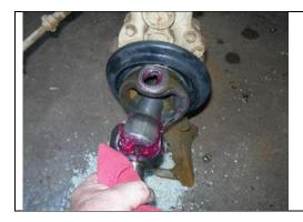
Next, install the axle. Don't forget the spacer on the inner axle. I have packed the joint with grease.
