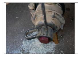
Install the two brass plugs into the lifting shackle.
