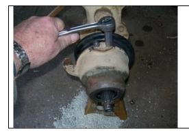
Pack the kingpin bearings with grease just like a wheel bearing and then install the bearings, hub and kingpins in the reverse order that you removed them. You can see that I've already installed the new hub seal in the knuckle housing.
