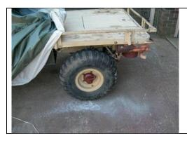
Service the knuckle with SAE 90 wt as per LO 9-2320-246-12, install the wheel and tire and you're ready to roll.
