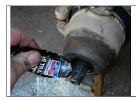
I like to put just a little sealant on the axle splines before I install the hub.
