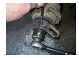
I snug the nut down, then use my small punch to align the holes in the nut and the axle.
