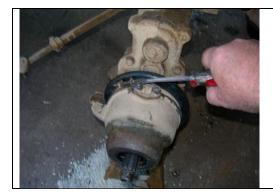
Install the band on the boot at the knuckle, make sure you have the band on the rubber and not on the edge of the knuckle housing, and tighten. Again, don't overtighten. Keep the screw and nut near the top of the knuckle where the boot does not flex as much.
