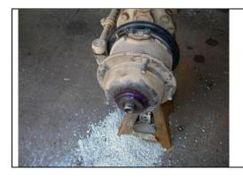
Install the hub onto the axle. You will have to work it gently until is slides all the way into the hub bearing. You can see that I've installed a new seal on the hub and greased it.
