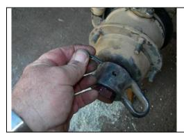
The lock pin is a 9/64" x 1 1/4" spring pin.
