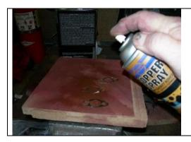
To keep oil from leaking around the kingpin shims, I coat each one with a spray Copper Cote sealant compound.
