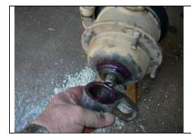
Install the lifting ring onto the hub, use plenty of grease or anti-seize compound.
