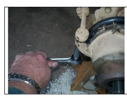
Install the tie rod with the nut and cotter pin.
