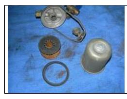
Here are the parts: the base and bail, the filter, the rubber gasket and the bowl.
