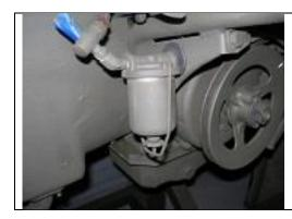
Unscrew the bail nut and remove the bowl. Twist the old filter off the base, the rubber gasket should come with it.
