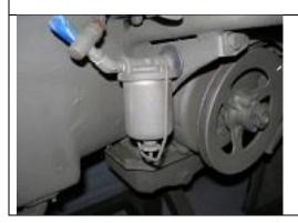
Install the bowl and the bail and tighten the bail nut. Hand-tight is enough, don't use pliers!
