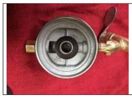
If you find this type filter on your mule and plan to replace it with the WIX 33034 filter, you must make sure that the smaller rubber seal is not stuck into the nub on the filter base or it will block the flow on the Wix filter.
