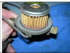
Twist the filter onto the "nub", paper-end in. It may take a little force to make the filter slip onto the "nub". Filter is a WIX 33034.
