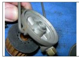
Make sure the base is clean, any silicone is scraped off and the rubber gasket is removed. The filter will fit onto the "nub" on the base.
