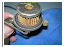
Now slip the rubber gasket over the filter and into the base. The gasket helps hold the filter into the base. On the mule, you can slip the gasket over the filter and then use the bowl to lift it into position on the base.
