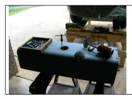
If you are finding lots of crap in your engine fuel filter, chances are, the in-tank filter is full of crap, too, and needs to be serviced. This will require that the tank be removed from the mule, and this opens up a whole 'nuther can of worms! (twisted-off screws on the pickup assembly, etc.)
