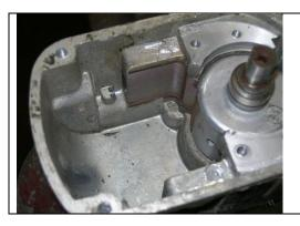
All the contact points inside the housing should be cleaned and polished. I use a wire brush in a Dremel tool, followed by a light scuffing with sand paper.
