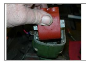
Remove the coil from the housing.
