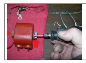
Don't forget to clean the contact points on the coil and the two coil retaining screws.
