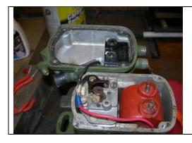
Reassemble the magneto, using a small amount of Loctite on the coil screws. Be sure to clean and polish the bottom of the point plate, even if you are installing new points.
