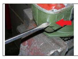
Remove the two coil retaining screws. You will have to use a little heat from a torch to get the Loctite to turn loose. Hold pressure on the screwdriver and add a little heat to the area shown by the arrow, and as soon as the screw starts to turn, remove the heat.
