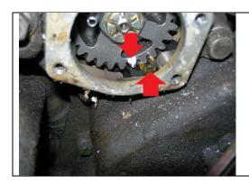
Install the magneto onto the engine. I like to retard the magneto by installing it one tooth to the left. Most engines seem run much better when they are timed this way, however, there are a few that don't like it at all, so you'll have to try it and see!
