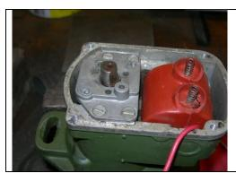
Now remove the 4 screws that hold the top plate to the magneto housing.
