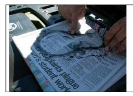
Once the correct clearances have been achieved, it's time to install the cover for the last time. A good coat of gasket sealer
