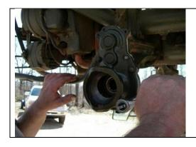
And install all the lock washers, nuts and bolts.
