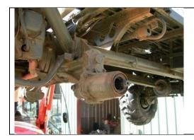
We removed the rear wheels, axle nuts and hubs. See the tutorial on dust boot replacement which explains how to remove the axle nut lock pins.
