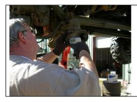
Next step was to remove the non-steerable drop housings from the rear axle.
