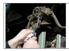
Time for lots of gasket scraping. These gaskets are tough, so be sure to remove all traces of the old gasket.
