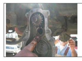
Inspect and grease the needle bearings.
