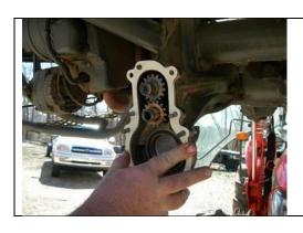
A new gasket is installed.
