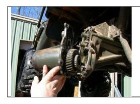
Watch the axle drive gear when you remove the housing, don't let it fall on your toe!
