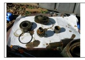
Here are the parts we will be reusing; the wheel bearing and lock ring, the drive gear and idler gear, and the axle spacer
