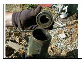
In our case, we needed to reuse several parts from the old 2-ws hubs. This shows removing the wheel bearing.
