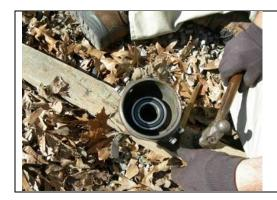
The old wheel bearings are installed into the steerable knuckles.
