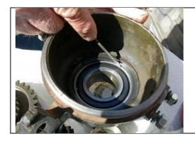
And the spiral lock rings are installed.
