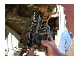
And the new cover is installed. We had some trouble here, sharp eyes will notice that the dowel pins are in the axle housing and also in the cover! It took us a few minutes to figure this out! Install several nuts and bolts and then check the clearance on the axle drive gear. This procedure is described in TM 9-2320-246-34 on page 5-22 and should not be skipped.
