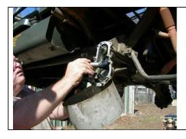
Cleaning and inspecting the bearings.
