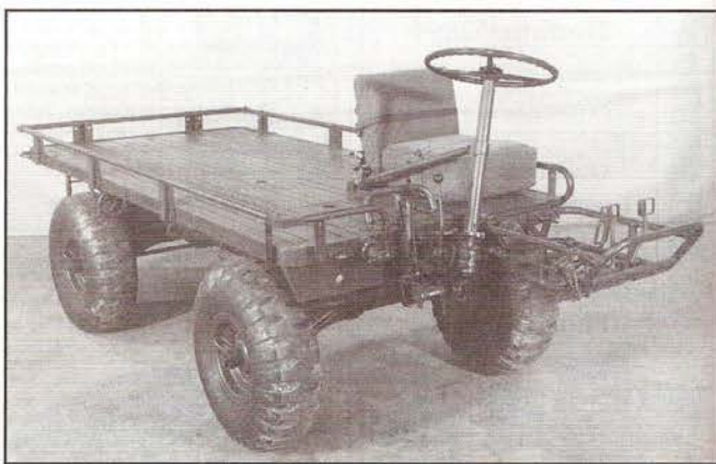
Figure 3. Shown above is one of the 3,609 M274A2s built by Bowen-McLaughlin-York between 1964 and 1967. The company only produced the 4-wheel steering version of the vehicle. Patton Museum, Fort Knox, Kentucky
