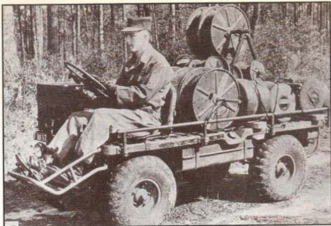
Figure 4. The Mule was a compact, versatile vehicle, and popular with the troops. Shown above is one fitted with cable reels for signals use. U.S. Army photo
