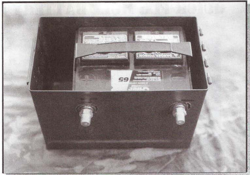
Two holes cut into an ammo can for the Squad Automatic Weapon provide clearance for the terminals of the side post battery. Battery can still be charged while in the can.
