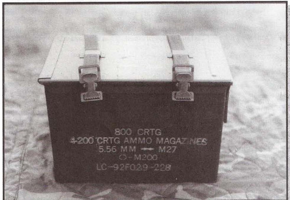
View of the completed ammo can/battery box arrangement from the outside, no battery terminals or cables will show once it is installed and the 1" web straps match the one used on the Mule's driver seat.
