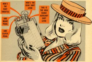
Put the auxiliary shift lever forward for high-range, depress your clutch, engage your conventional transmission in low gear and drive off-same as any other vehicle.
