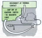
You can either disconnect 'em (the cable) from the thermal contact and snip the cable off at the junction where it got spliced to the ignition switch-to-magneto cable...
