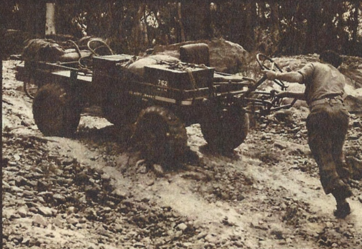
CONTROLS swing out so vehicle can be driven while walking or crawling behind — handy if advancing under fire.
